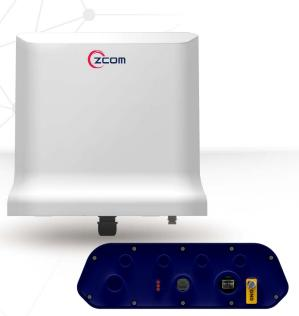
SP420-F 802.11ac Wave 2 4x4 dual band outdoor access point is with Multiple-Input Multiple-Output (MIMO) technology, provides a data rate of up to 2.3Gbps, and can accommodate up to 512 wireless devices.
